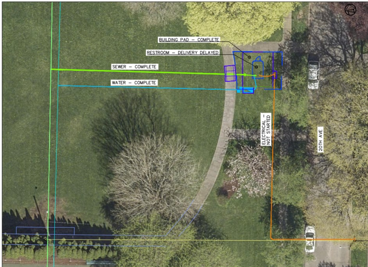
Figure c - Current restroom location and utility work progress.
